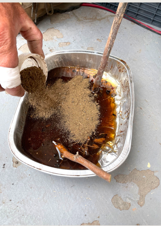
Ground deer droppings and other additives like red ochre in this version are mixed in while resin is hot.
