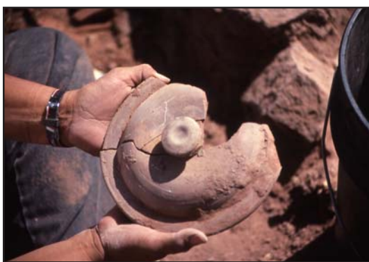
Top: Melted inner faces of kiln bricks. Bottom: A misfired crock lid.
