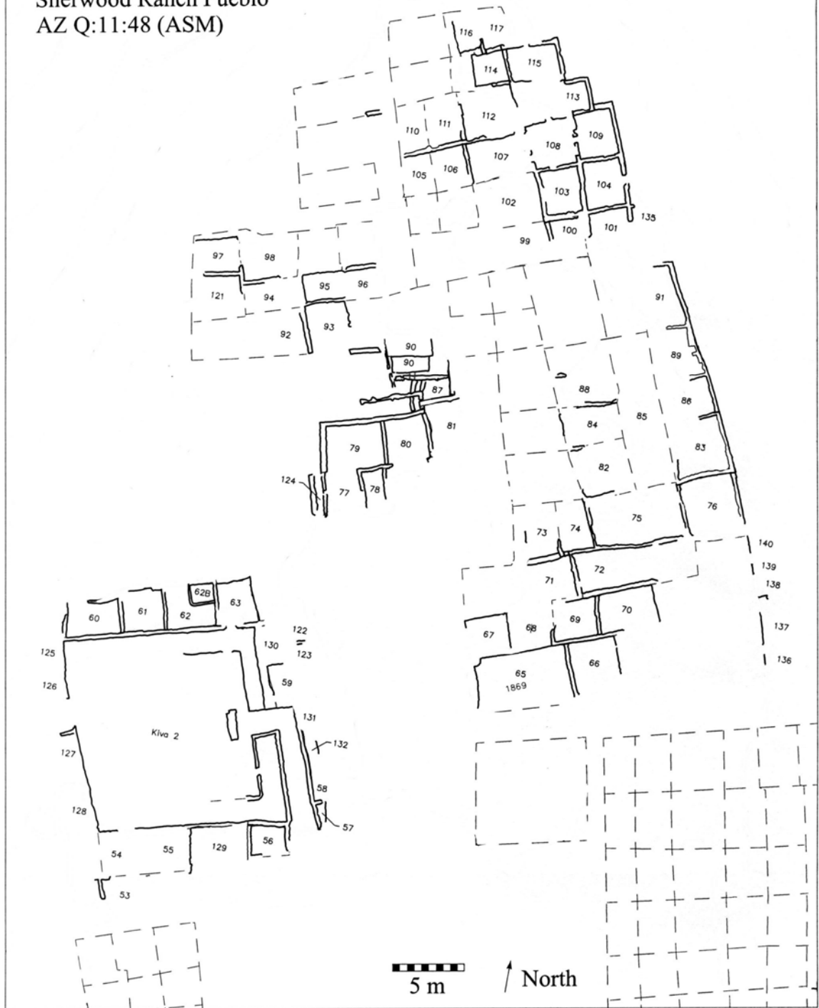
Figure 6.1 Plan of Northern pueblo highlighting abutment and bonding relationships for known architecture.
