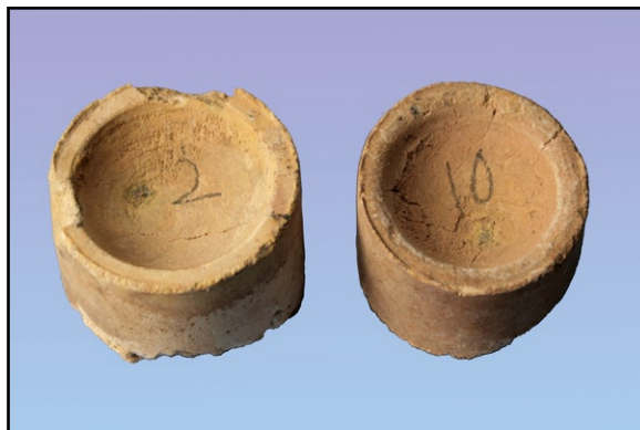
Top: Three views of a decorative Mexican duck. Bottom: A pair of cupels, used by the Tucson Sampling Works to assay ores, marked in pencil with sample numbers "2" and "10."
