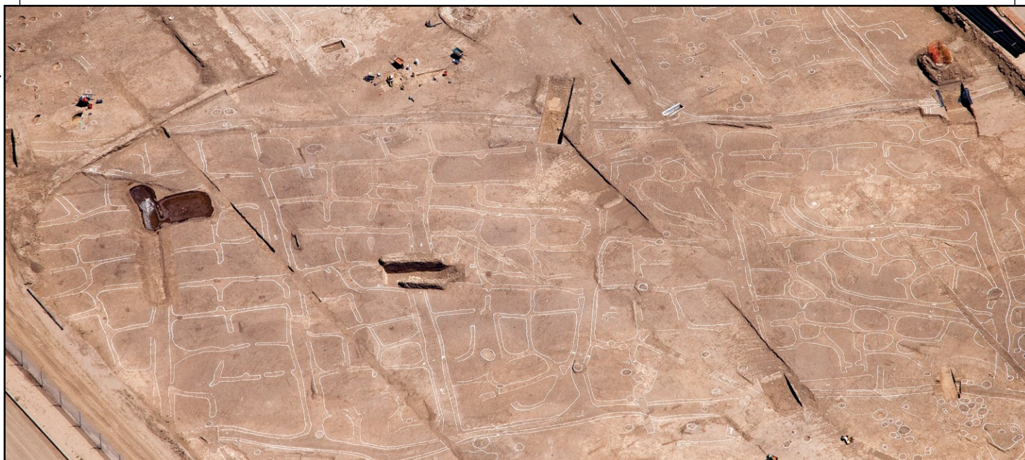
Aerial view of recently documented fields from 1200 B.C. at the site of Las Capas on Tucson’s north side. The main canal tapped the Santa Cruz River, and secondary ditches diverged from the main canal and then delivered water to tertiary ditches that watered individual bordered fields. Secondary ditches are visible at the bottom and close to the top of this photograph. They carried water from the right toward the left side of the image, and water was then diverted into the tertiary ditches (oriented from bottom to top in this image). Distance across this image is approximately 240 feet.
